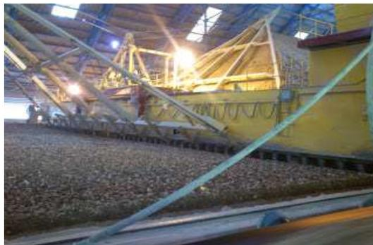
Gambar 3.4 *Reclaiming Scraper*
