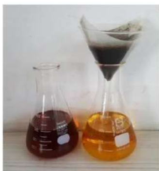
Figure 8. Hot mud adsorbent testing on waste cooking oil
