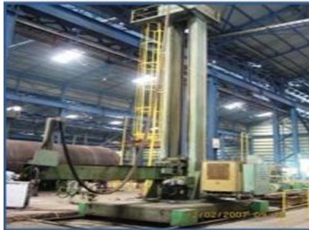
Gambar 3.7 Pengelasan Manipulator & Boom SAW
