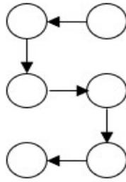
Gambar 2.7 Pola Aliran Bahan Zig-Zag (*S-Shape*)
