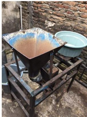
**Gambar 7.** Mesin Giling Tempe
