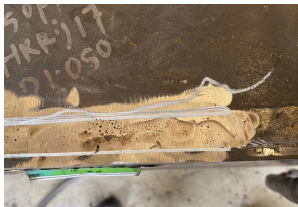
Gambar 2.5 Cacat Pengelasan Porositas ( Porosity )
