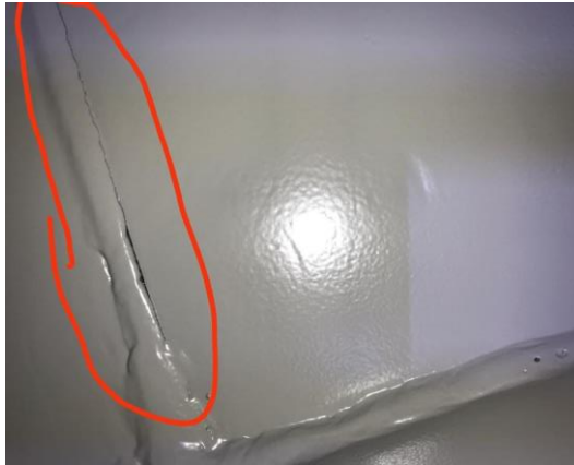
Gambar 2.7 Cacat Pengelasan Overlap (Kelebihan Elektroda)
