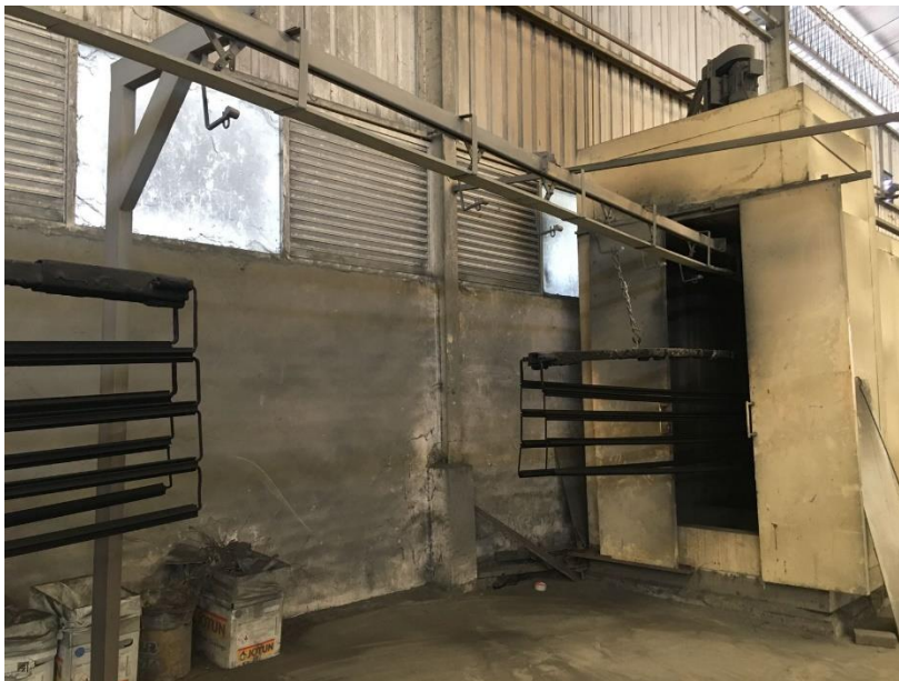
Lampiran 13 : Pengering Alumunium
