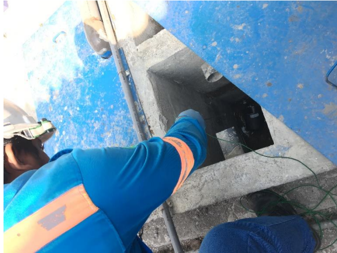
Gambar 5.1 Proses Pengambilan Air Sampling Limbah Domestik PT. PAL Indonesia (Persero)
