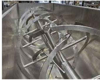
**Gambar II.2** *Silinder Mixing Horizontal*
