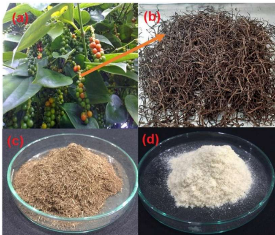
Fig. 1. Images of (a) pepper tree, (b) dried pepper stalk fibers, (c) pepper stalk powder after milling and (d) PW Cellulose.
