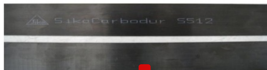
Figure 12. CFRP plate size 1.20 X 50.00 X 1000 mm
