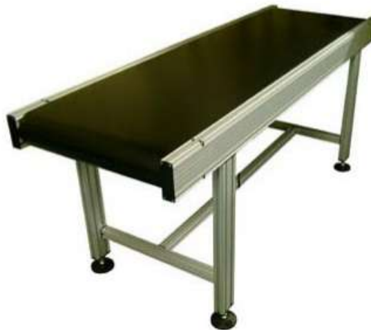
Gambar 2.21. Bentuk flat belt conveyor.
