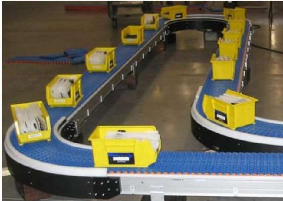
Gambar 2.26. Wide Plastic Belt conveyor membawa material berupa benda.
