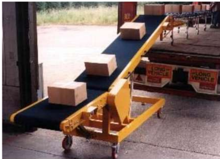
Gambar 2.28. Gravity Belt conveyor.
