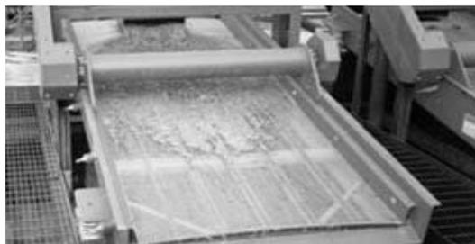
*Gambar 2. 4 Inclined Screen*
