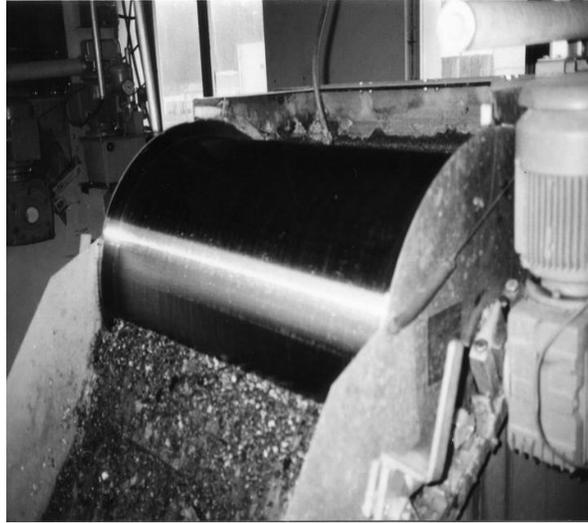
*Gambar 2. 5 Rotary Drum Screen*
