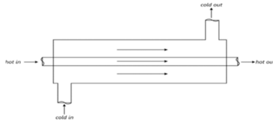
Gambar II.12 Arah aliran co-current/paralel flow
