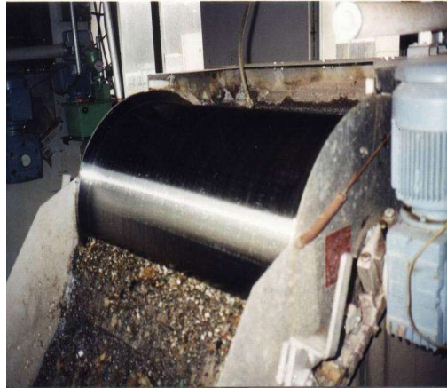
Gambar 2. 7 Rotary Drum Fine Screens (Sumber: Irman, 2015)
