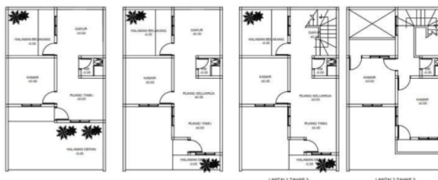
Figure 4. House plans of type 21m 2 growth with 60m 2 land area (from left to right: stage 1,2,3)
