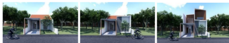
Figure 7. Front view of a house growing type 21m 2 with a land area of 72m 2 (from left to right: stage 1,2,3)
