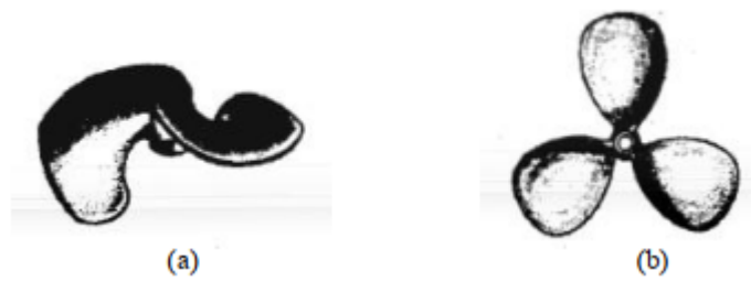
Gambar 2.11 Tipe Propeller (a) Propeller 2 blade, (b) Propeller 3 blade
