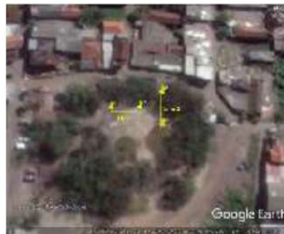
Fig.4. Acquisition design of resistivity survey
